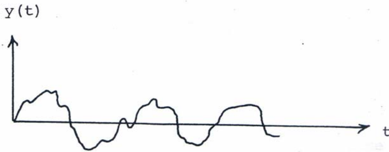
Figure 2-1-b The Random Signal subtracted from a Sine Signal. The average zero crossings \approx \frac{2}{T} when the amplitude of the Sine Wave is large.
