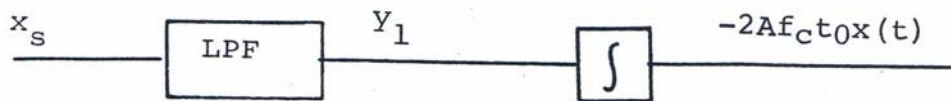
Figure 4-8. The Reconstruction of the Base Band Signal from the Train of Bipolar Impulses
